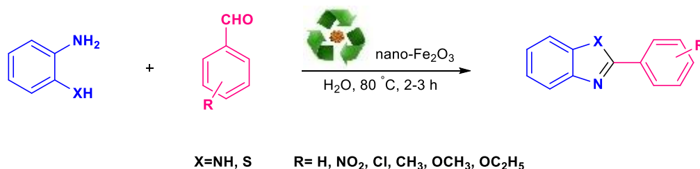
Scheme 9: Synthesis of benzimidazole/benzothiazole derivatives
